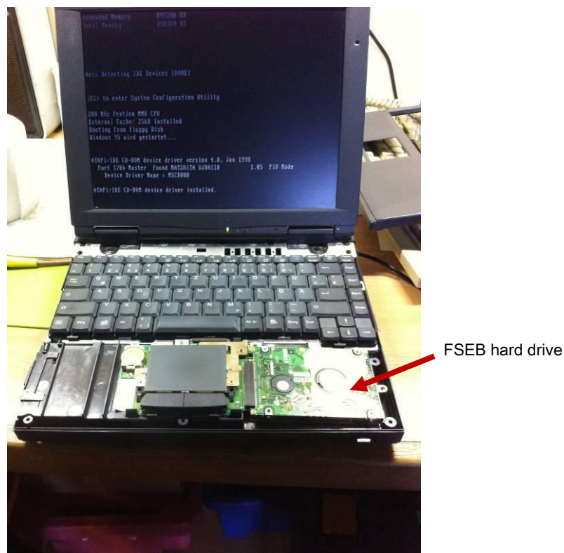
Figure 13: old laptop with built-in hard drive FSEB
