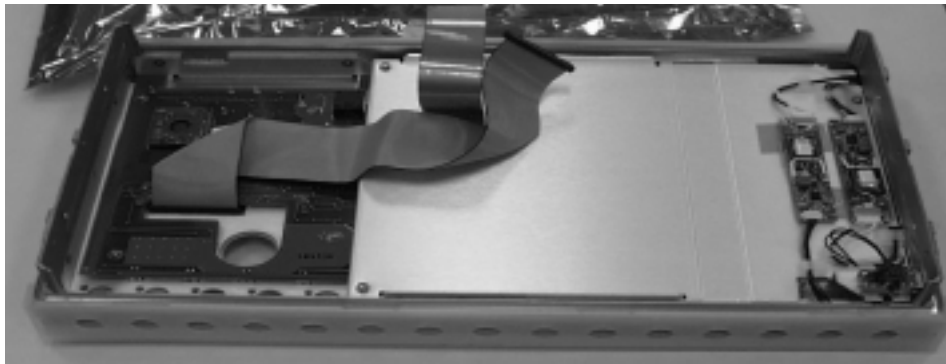
The back of the 86140A/B, 86141B, and 86142A/B front panel assembly
