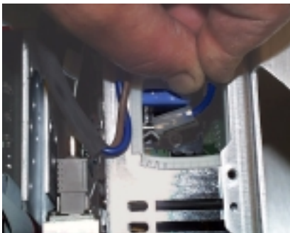
Figure 3-26. Disconnecting the line module power connector from the power supply
