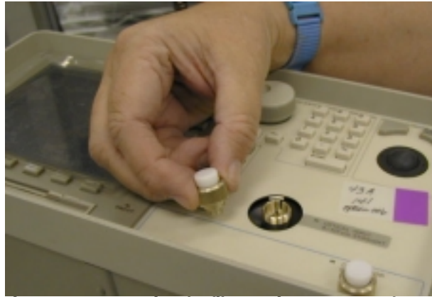
Figure 3-20. Removing the fiber-optic connector adapters
