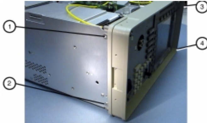
Figure 3-22. Attaching the front panel to the chassis
