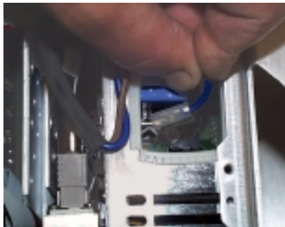
Figure 3-53. Disconnecting the line module power connector from the power supply
