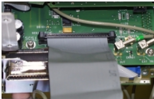
Figure 3-28. Disconnecting the hard drive ribbon cable from the mezzanine board
