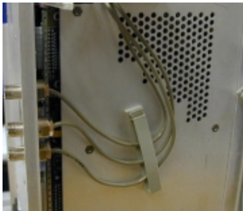
Figure 3-25. Removing the cables from the cable clamp
