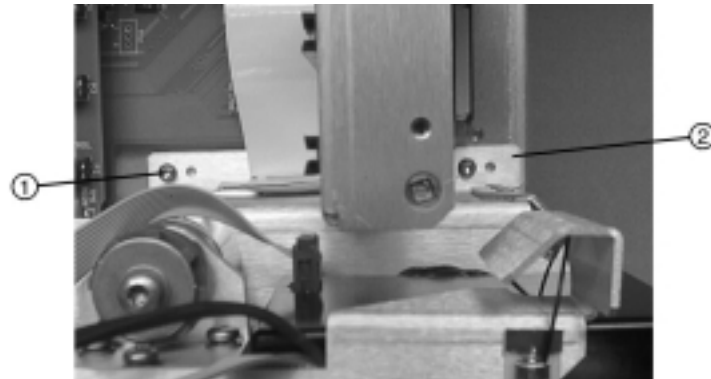
Figure 3-71. Removing the screws fastening the optical assembly to the rear panel
