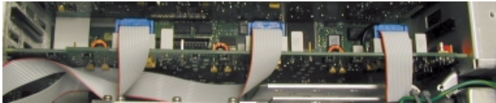
Figure 3-13. Disconnecting the connections on the Options board
