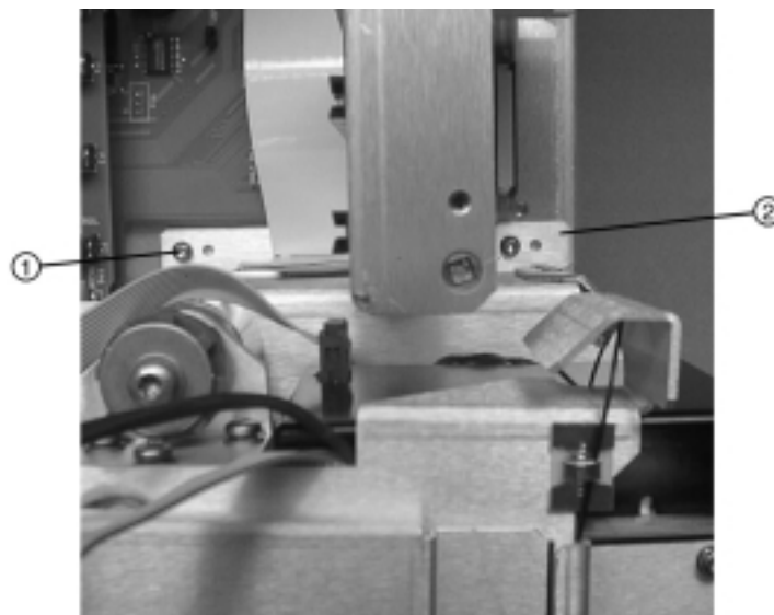
Figure 3-65. Removing the screws fastening the optical assembly to the rear panel
