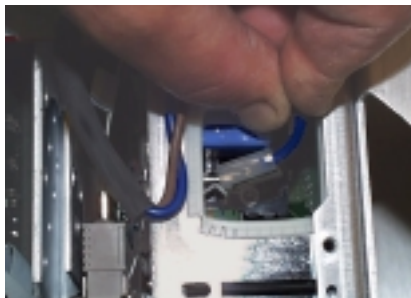
Figure 3-57. Disconnecting the line module power connector from the power supply
