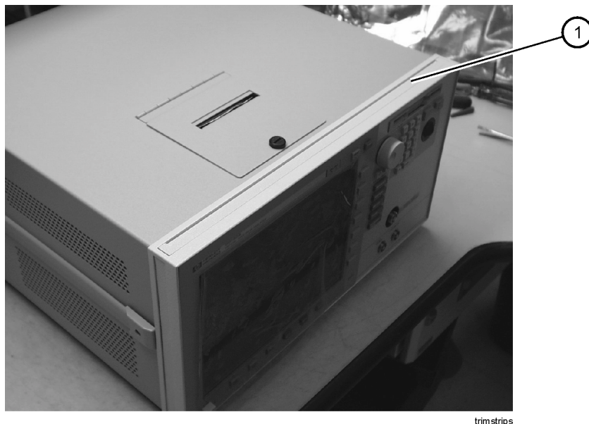
Figure 3-15. Removing the trim strips from the front panel assembly
