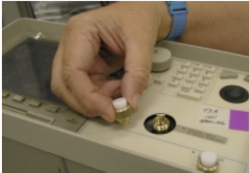
Figure 3-14. Removing the fiber-optic connector adapters
