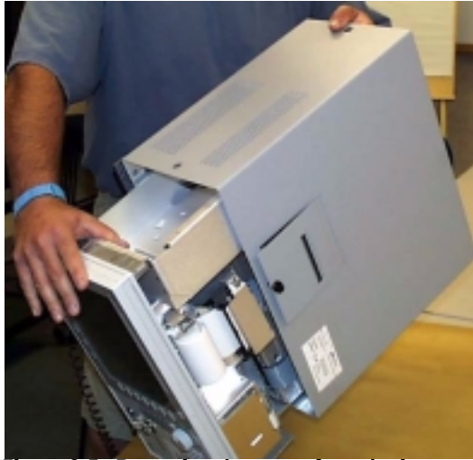
Figure 3-5. Removing the cover from the instrument
