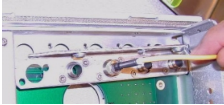
Figure 3-18. Removing the connectors (Left - Early model, Right - with new bracket assembly)
