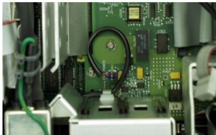
Figure 3-29. Disconnecting the fan connector from the mezzanine board
